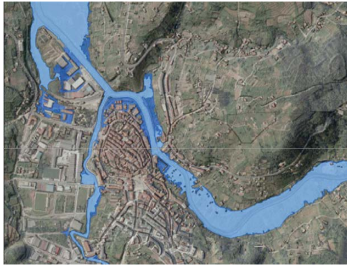
Figure 3. Inundation maps for the return period of 2.3 years (from Sopelana et al. 2018).
