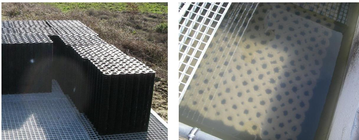
Figure 2 Structured packed rigid media (BIO-NET). Left: clear media. Right: biofilm developed on media after elapsed time 8 days of operation (SAF-1 cell)
