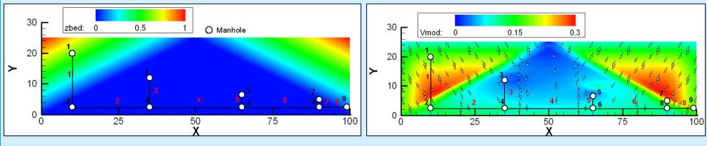
**Figure 5**. Basin topography in meters (left) and velocity field in m/s (right)
