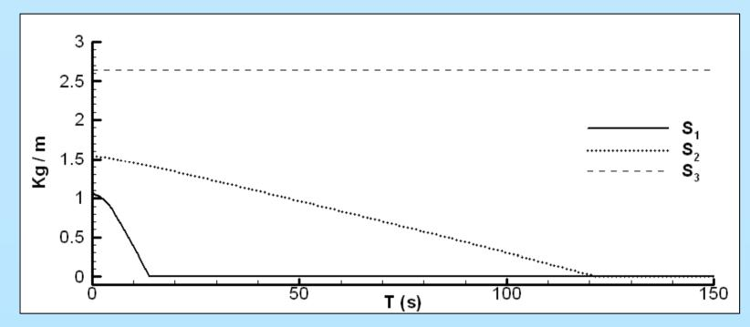
Figure 7. Sediment concentration versus time for the three considered sediment types.
