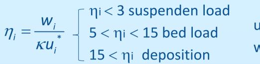
u\* -> shear velocity w -> settling velocity
